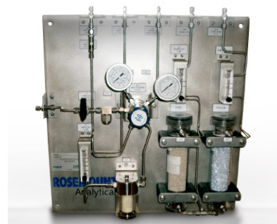
Figure 1 - External Sample Handling System
