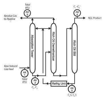
The stripping oil plus any of the heavy components from the natural gas enter the rich oil still where the natural gas liquids are boiled out of the stripping oil. This natural gas liquids product stream is then sent to a natural gas liquids plant for further separation or is sold to a chemical plant as feedstock.
