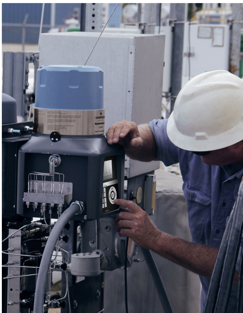
Figure 2. Basic natural gas analysis can be covered by a C6+ analyser, such as Emerson's Rosemount™ 370XA Gas Chromatograph. Its enclosure permits field mounting in most areas classified as hazardous.
