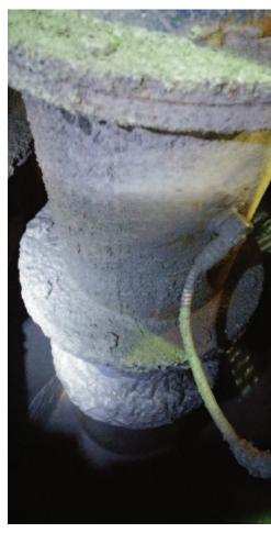
n 2014, Copper Mountain Mining Corporation decided it wanted to optimize its 35,000 tonne-per-day copper mine in British Columbia and exceed its nameplate capacity. Therefore, it began moving high tonnages of coarse material through its ball mills. However, this inevitably resulted in plugging and roping incidents with its cyclones at an average of three or four per week, causing downstream interruptions in the flotation circuit.
