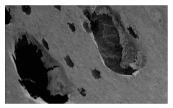
*Figure 1b.* This SEM image at 20X reveals the localized attack of the hydrochloric acid. For high concentrations of hydrochloric acid, tantalum is compatible.
