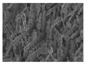
*Figure 2b.* This SEM image at 80X reveals the dendritic structure within one of the colonies. The molybdenum-rich regions have been preferentially corroded away deep inside the casting. For nitric acid, CF-3 (304L cast equivalent) without the molybdenum is compatible.
