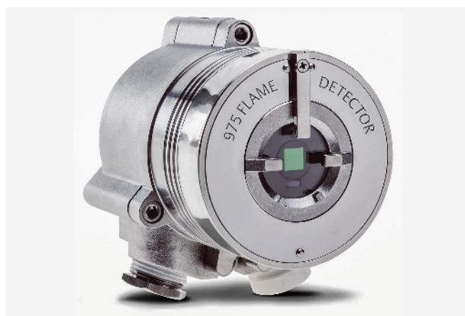
FIG. 1. Flame detectors are typically designed to sense specific radiation wavelengths produced by burning hydrocarbons and/or burning hydrogen. This tuned sensitivity helps avoid false alarms. Photo courtesy of Emerson.
