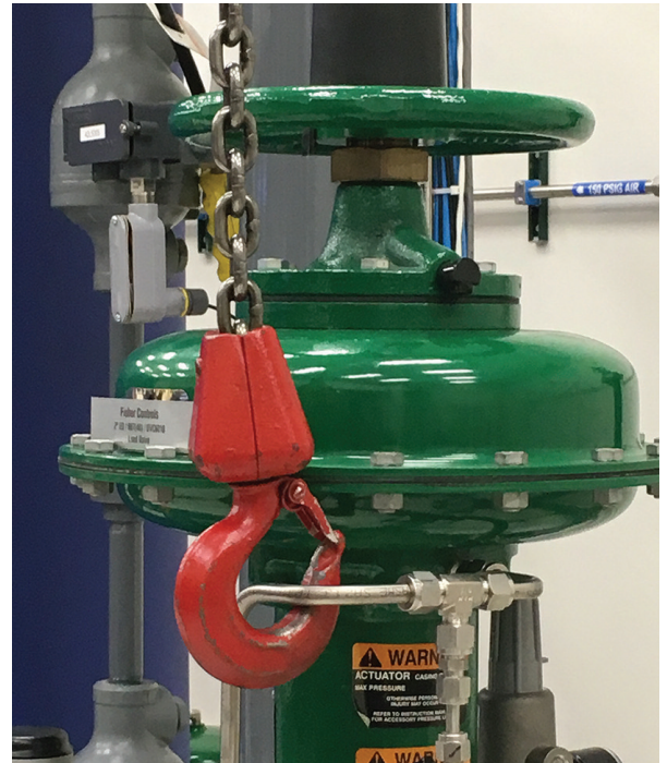
Figure 1: External instrument tubing on a control valve can be easily damaged by improper use – such as picking up the valve by the tubing line
