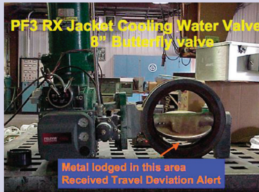
Fig. 2. Without a travel deviation alert, this control valve would not have been checked and problems not identified until too late.
