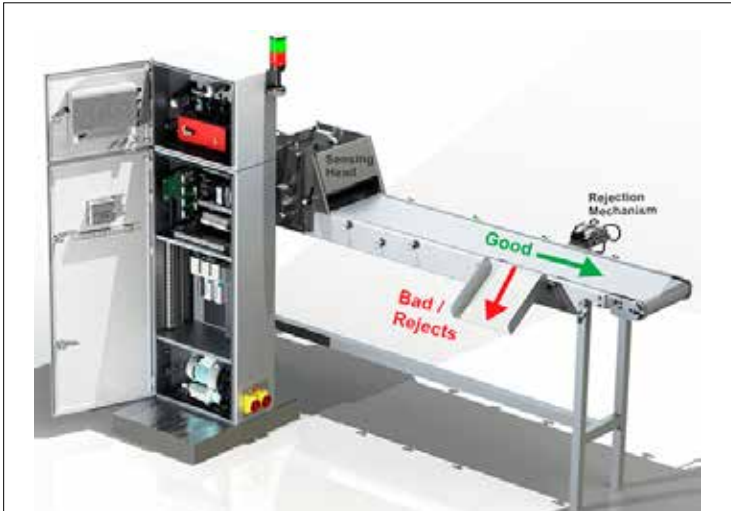
Figure 4: The system is self-contained and can be connected to a rejection device mounted on the conveyor. Photo courtesy of Emerson.
