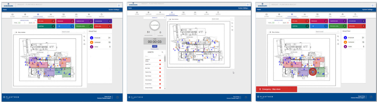
Figure 1. Software designed to support location system functions can include pre-designed user graphics, including geofencing (left), safety mustering (middle), and safety alerts (right).
