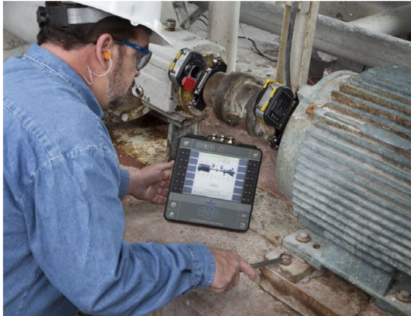
This multi-purpose machinery analyzer includes laser shaft alignment capability.
