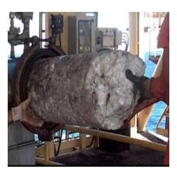
Hydrate Formation Source: Giarvarini, C. & Hester, K. (2011). Gas Hydrates. p. 98. and corrosion, owner-operators and service companies inject appropriate chemicals into oil or gas wells. Managing flow assurance issues such as these is critical, since they can cost the oil & gas industry billions of dollars in repairs and maintenance. According to NACE International, corrosion alone costs the US upstream oil & gas industry an estimated \$1.4 billion every year.
