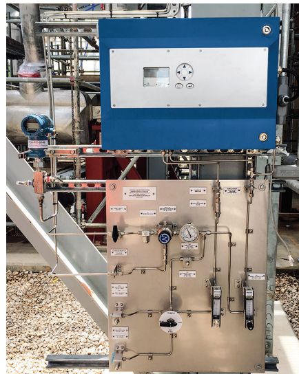
FIG. 3. Conventional continuous gas analyzers are often used for process control, product optimization and emissions monitoring.
