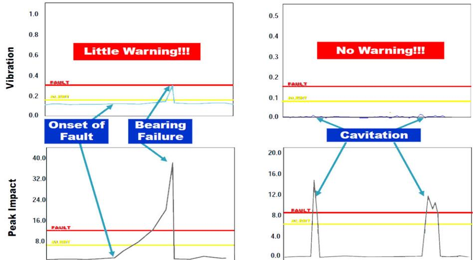
**Figure 2.** What is Peak Impact Detection? Both Overall Vibration and PeakVue are shown. The peak value is extracted from very fast sampling at 50,000 times per second. The PeakVue measurement detects the micro-burst that occur when metal impacts metal inside the machine. PeakVue represents the peak value of these impacts.
