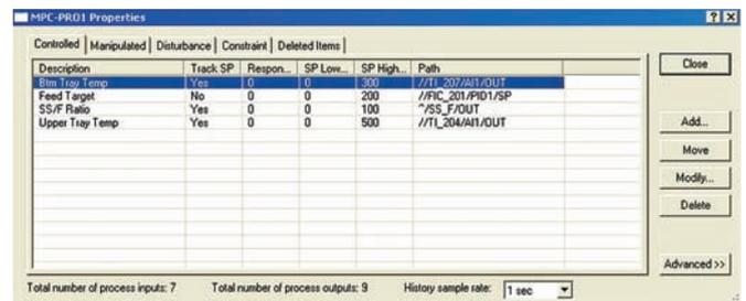
**FIG. 4** Embedded MPC configuration can be easily edited to accommodate the specific project needs.
