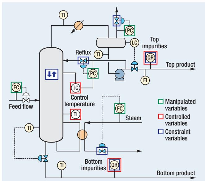
**FIG. 2** Advanced control of distillation columns like this one can be generalized from one site to the next.
