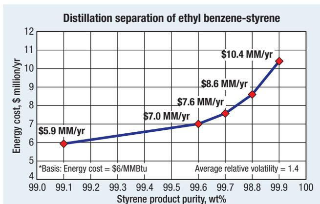
**FIG. 1** Energy cost vs. product purity in a styrene column.<sup>3</sup>
