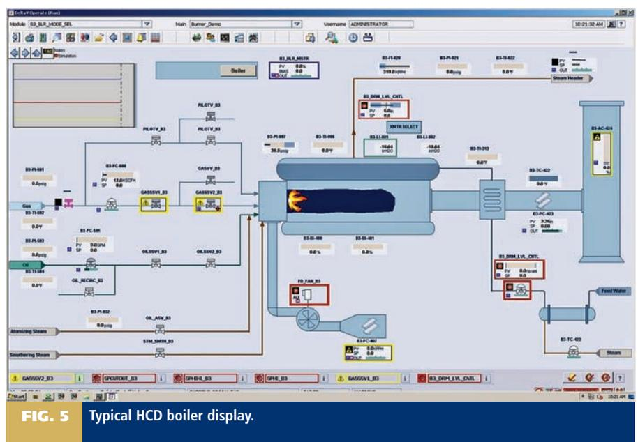
**FIG. 5** Typical HCD boiler display.
