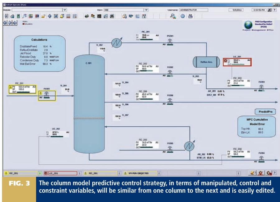
**FIG. 3** The column model predictive control strategy, in terms of manipulated, control and constraint variables, will be similar from one column to the next and is easily edited.
