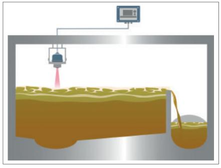
> The latest non-contacting radar transmitters provide an accurate, reliable and cost-effective level and flow measurement solution in combined sewer overflow applications.
