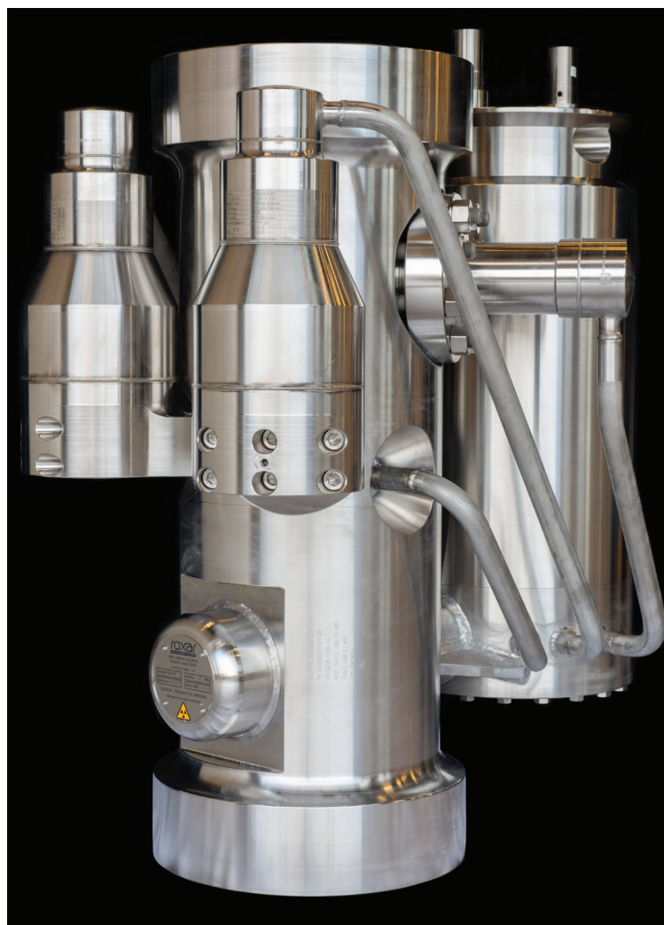
FIGURE 3. The Roxar subsea Wetgas meter measures the total water content in the gas to provide individual flow rates of gas, condensate/oil and water. (Source: Emerson Automation Solutions)
