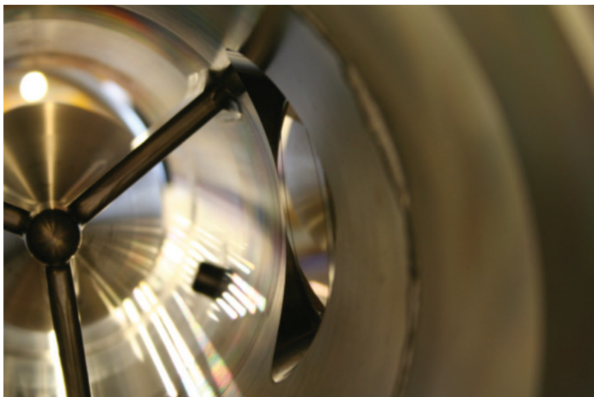
FIGURE 1. The salinity sensor is integrated into the meter. (Source: Emerson Automation Solutions)
