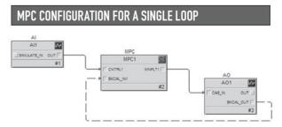
Figure 1. Model predictive control (MPC) can be used to effectively control a single input, single output (SISO) process that is dead-time-dominant, where PID may not provide satisfactory performance.
