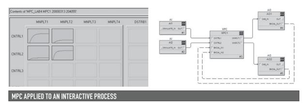
Figure 2. I: In an interactive process where a change in one manipulated input may impact multiple controlled outputs, the common workaround is detuning the PID controller. Instead, the interaction can be addressed by a single MPC block.
