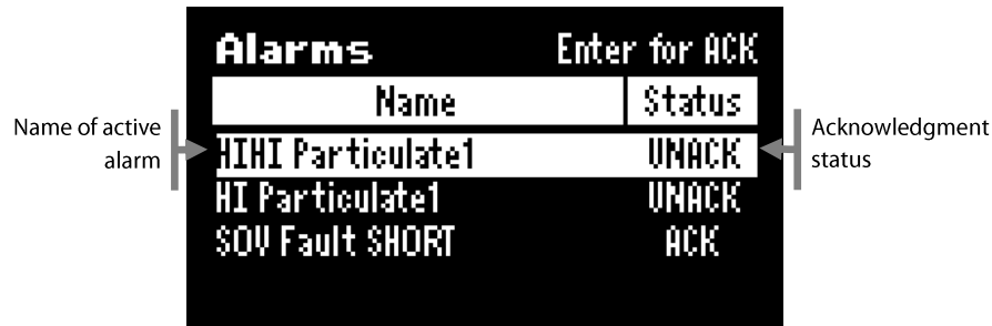
Active Alarms Screen
