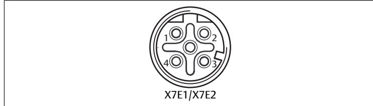
Fig. 3: Fieldbus connection pin assignments
