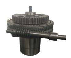
Smooth gearing is achieved with an all-metal, internally-located, greased, and self-locking epicyclical gearing system, which helps eliminate the need for motor brakes.
