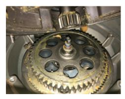
Robust materials are selected for loaded parts; for example, sintered alloy epicyclical gearing and cast-iron output drives.
