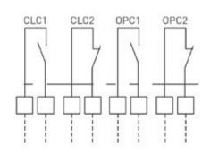
Four latched-type output contacts are available for remote indication of fully open or closed status. Output contacts for monitoring and blinker/local selector indication are also available.
