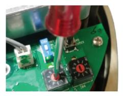
Easy configuration via two rotary switches on the logic board to configure each function, which includes position, torque, open/close speed, reverse mode (clockwise/counter-clockwise) and output contacts.
