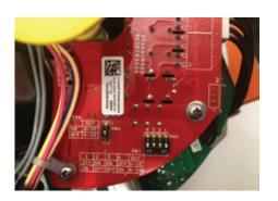
OM1: input/output module offers analog positioning control and position feedback, 4 additional SPST output contacts (configurable) independently settable at 10 points along the stroke, information about loss of input signal, and a local selector position alarm (with OM3 installed).
