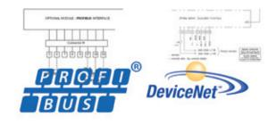
Simple connection to a bus system is possible with the optional OM9 (PROFIBUS DPV0/V1) and OM11 (DeviceNet) communication cards.
