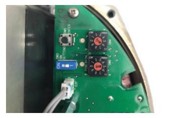
Precise torque control is configurable via user-friendly rotary switches located inside the control enclosure; bi-directional torque values of 50%, 75%, and 100% of nominal torque may be selected.
