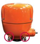
Mechanical travel stops at the base of the enclosure prevent over-travel during operation with the handwheel or motor, providing  $\pm 10^{\circ}$  of over/under travel in each direction (resulting in 70° minimum and 110° maximum angular stroke).
