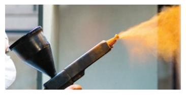
Electrostatic powder coating provides protection from the elements.
