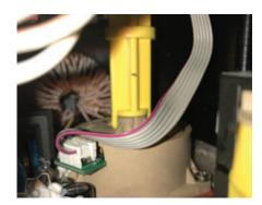
Absolute position sensor covers 110° of rotation, with travel endpoints set by the rotary switch (standard)
