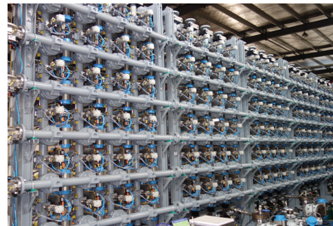
A 3 inch manifold with 36 inlets and 12 outlets undergoing Factory Acceptance Testing.
