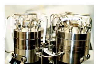
The Rosemount 700XA Gas Chromatograph has the capacity to support up to 6 analytical valves, which are quaranteed for the life of the system.
