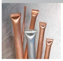
Ultraseal ultrasonic systems hermetically seal copper and aluminum tubes. A one-step operation crimps, seals and cuts off charged tubes in under one second. Systems are suited to automation for high levels of efficiency and productivity.
