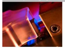
Ultrasplice systems ensure precision splicing of non-ferrous wires in a wide range of sizes. Ultrasonic splicing results in a superior electrical connection over crimping, soldering or resistance welding and offers savings in power consumption, elimination of consumables and long tool life.
