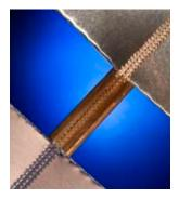
Welding variables can be precisely monitored and controlled to provide consistent results. The extremely versatile Ultraseam systems, when operated at 20, 30, 40 or 60kHz, function as a high-precision continuous seam welding system. They are the perfect machines for facilities that can benefit from the systems' flexible and space-saving design.
