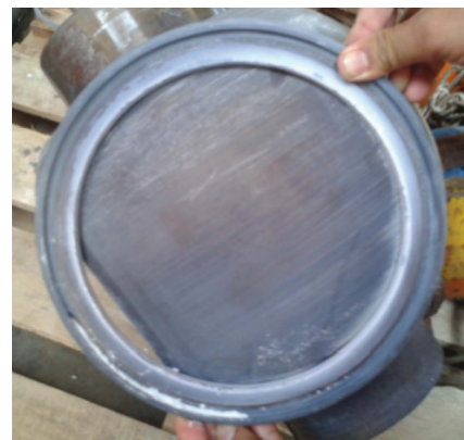
FIGURE 3 Conventional ball valve on abrasive dust service
