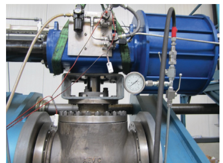
FIGURE 7 Switching valve with low emission packing undergoes testing
