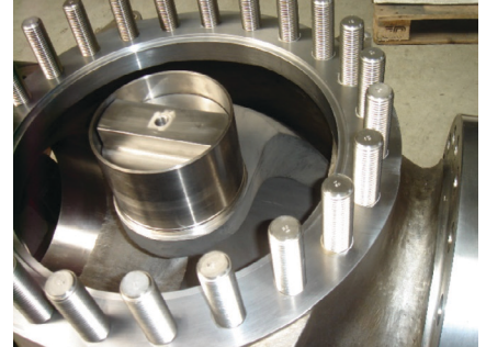
FIGURE 5 Chromium carbide coated ball
