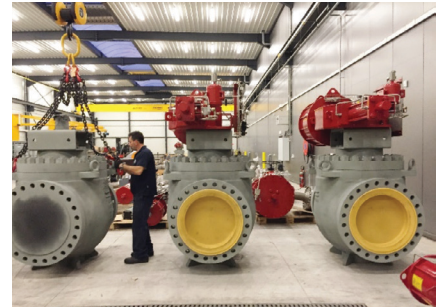
FIGURE 6 Modern rotary switching valves
