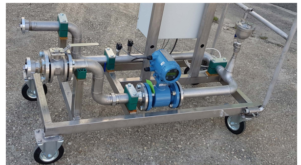
Emerson's Rosemount™ 8732E Magnetic Flow Meter Transmitter and Rosemount 8705 Flanged Magnetic Flow Meter Sensor
