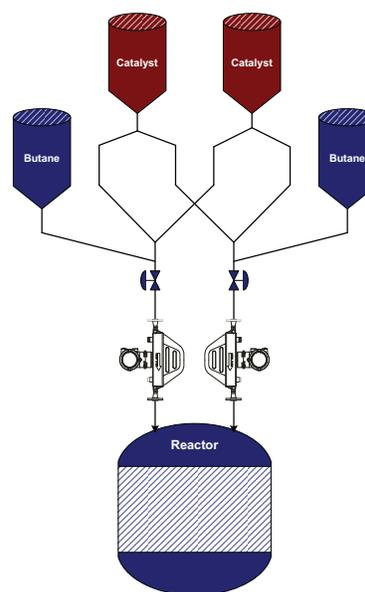
*Micro Motion F-Series meters on catalyst feedline*
