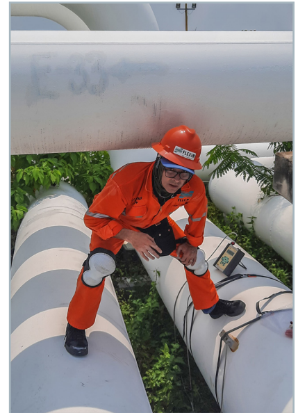
Eng. Fernando Sosa, Flexim's Regional Sales Manager Mexico, carrying out test measurements on a DN900 crude oil pipe.
