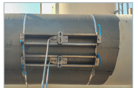
Powerful 0.5 MHz type K transducers are mounted parallel to each other on the pipe for NoiseTrek parallel beam (NTPB) measurement..
