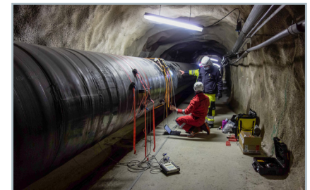
First, test measurements were carried out in order to determine the most suitable transducer type and the most appropriate transducer arrangement.
