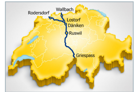
The Transitgas transport system consists of 292 km of natural gas pipeline with several tunnels, a compressor station with waste heat recovery systems, a measuring station, and various valve stations.
