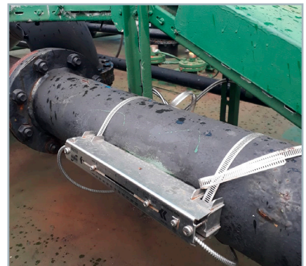
Measuring point with clamp-on ultrasonic transducers installed in Variofix L mounting system.
