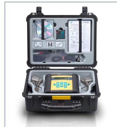
A complete measuring system, compact in its rugged case: The portable and battery-powered FLUXUS® G608 with clamp-on ultrasonic transducers and all necessary accessories.
