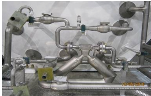
Micro Motion sensor mounted at the back of the LNG vehicle
