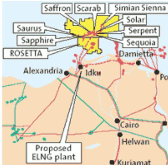
There are three principle fields in the WDDM concession: the Simian/Sienna field and the Sapphire field which is tied back to the Scarab/Saffron field. From the Scarab/Saffron field the gas is commingled before transferred to Burullus' onshore processing facilities at Idku near Alexandria.
