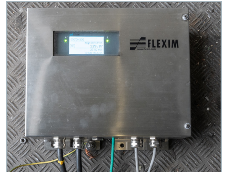
The stationary FLUXUS® G722 ST-HT ultrasonic system is used as a measuring transmitter.
