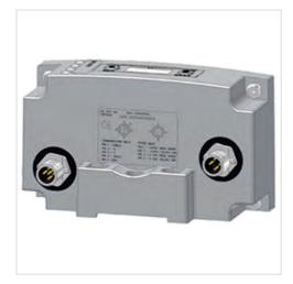
Version Bus coupler -10 ... 50 °C Ambient temperature min./max. 24 V DC Operational voltage electronics -10% / +10% Electronics voltage tolerance Power consumption electronics 0.1 A Operating voltage, actuators 24 V DC Total current for actuators 4 A IP65 Protection class Number of solenoid coils max. 32 Number of valve positions max. 32
