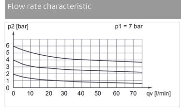
p1 = working pressure, p2 = secondary pressure, qv = nominal flow
