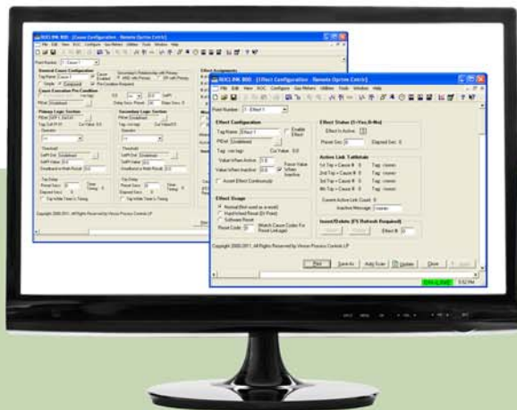
The configuration screens for Causes (rear) Effects (front)
