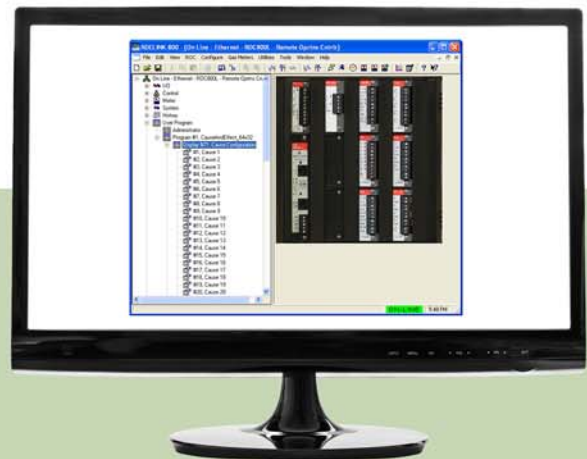
Multiple Causes shown in the ROCLINK™ 800 Configuration Tree
