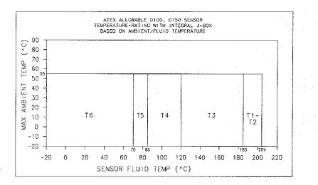
Note: Use the above graph to determine the temperature class for a given fluid and ambient temperature.
