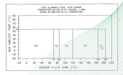
Note: Use the above graph to determine the temperature class for a given fluid and ambient temperature.
