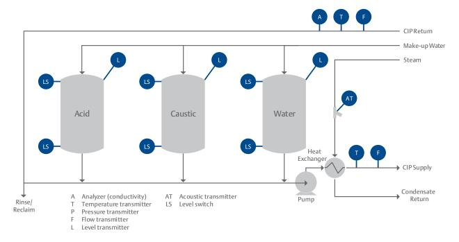
A typical CIP station design: the sytem is usually highly automated.
