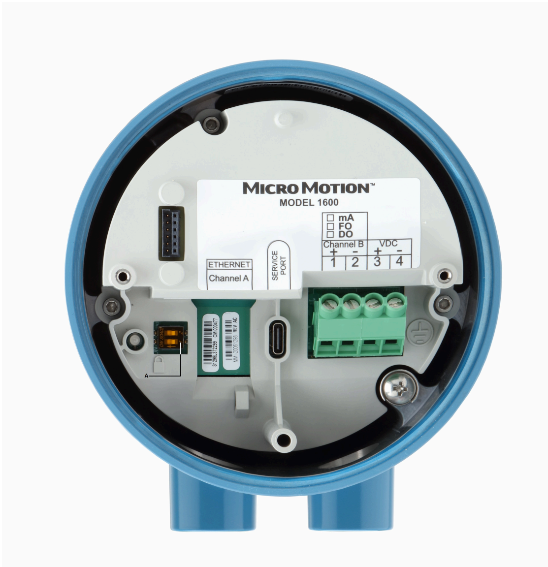
Figure 11-2: Setting Switch 1 ON (to the left) to Set Write-Protection
