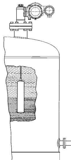
MONTAJE TÍPICO DEL SENSOR SIN JAULA
