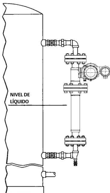
MONTAJE TÍPICO DEL SENSOR CON JAULA
