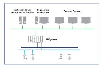
**The Operator Console (OC)** software element is used by the operator to monitor and control the process.
