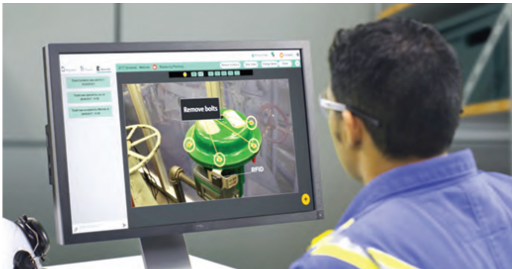
Figure 1: Remotely located expert seeing the problem in real time via field technician with wearable technology
