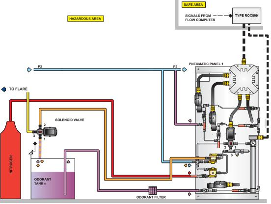
SUPPLIED BY SYSTEM INTEGRATOR \*ASCO SOLENOID PN #JBEF8320G140VDC12
