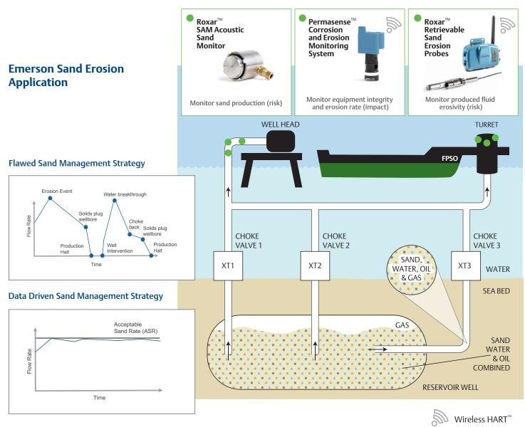
A Data Driven Sand Management Strategy increases production while keeping HSE conditions and facility integrity under control.
