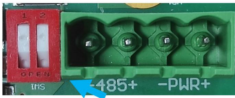
Figura 3-6: Resistor do terminal RS485
