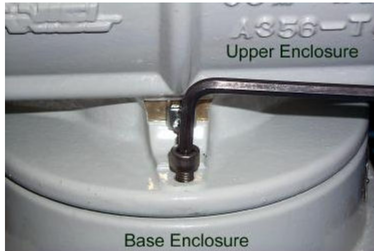
Figure 1-8: Remove Bolts from Base Enclosure Cover
