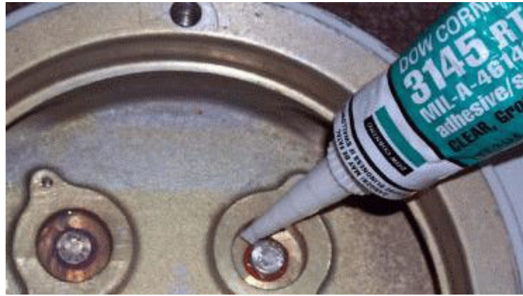
Figure 2-4: Apply RTV Sealant Around Bolts
