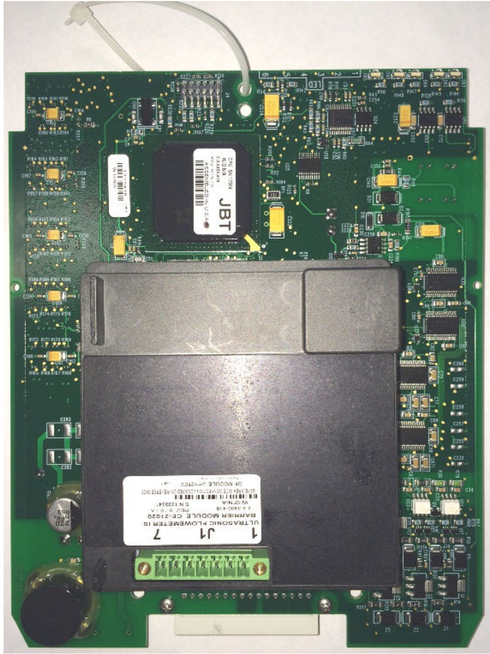
Figure 1-6: 3800 Series CPU Board with I.S. Barrier Board Piggy-Backed on CPU Board
