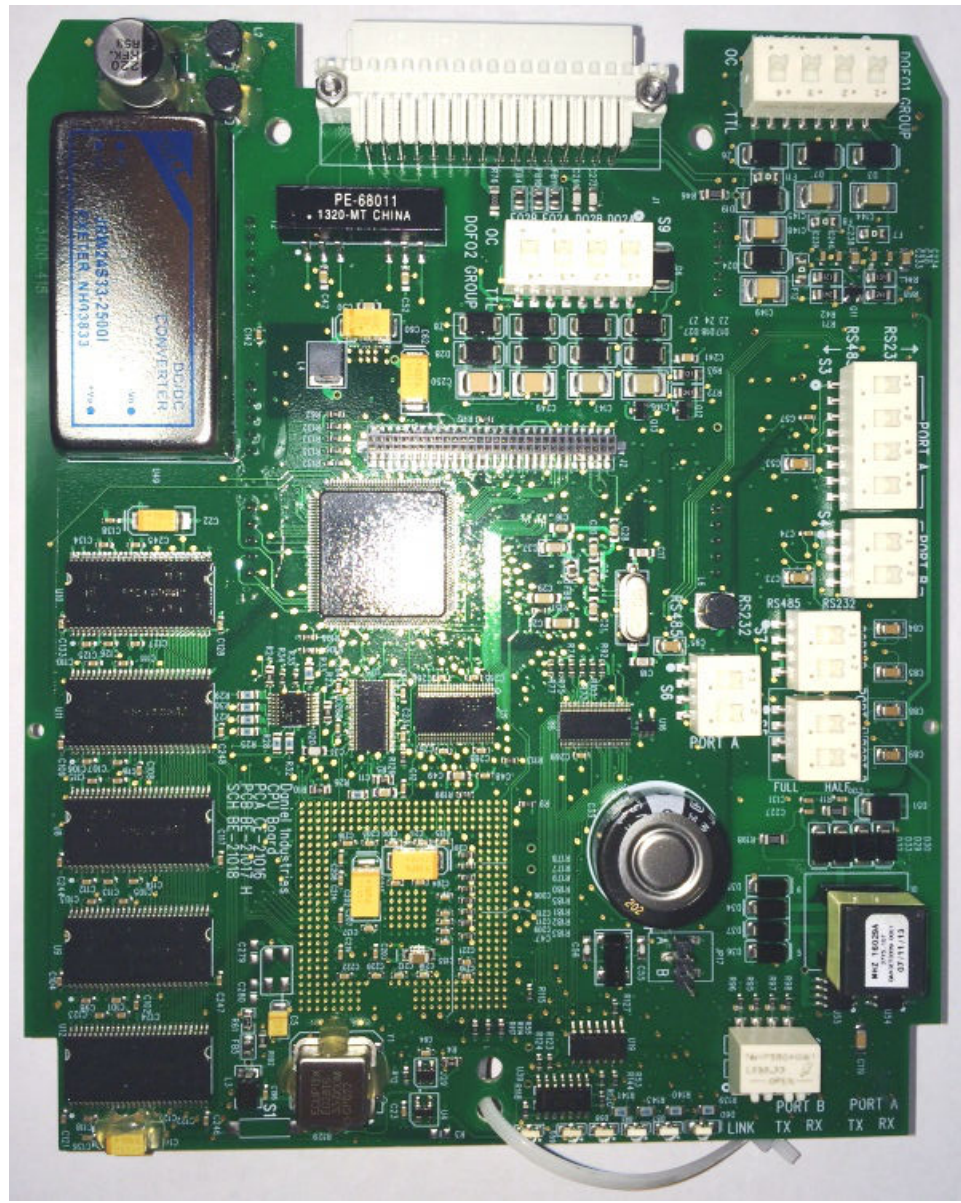
Figure 1-5: 3800 Series CPU Board Showing Switch Settings
