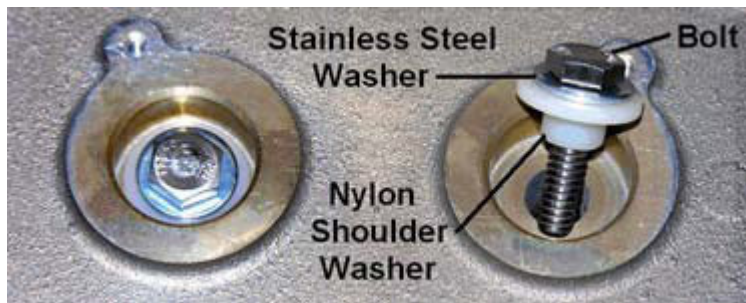
Figure 2-3: Insert ¼-in. Bolts
