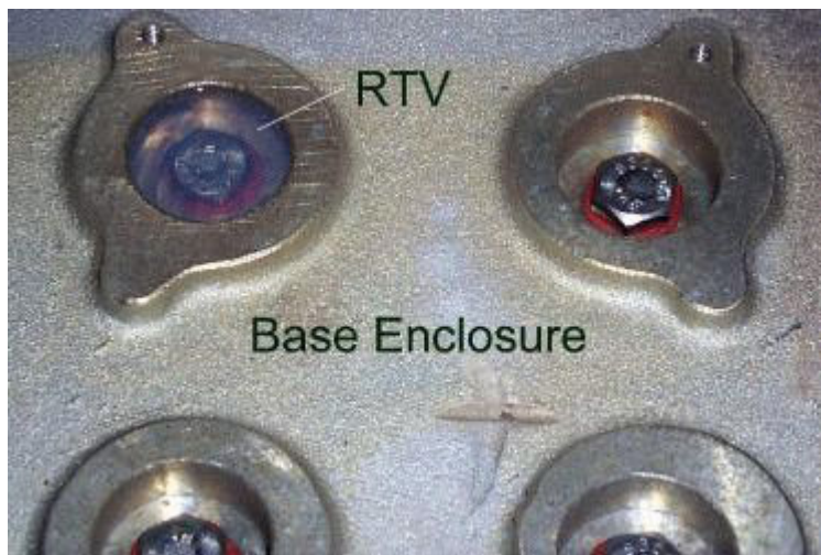
Figure 1-10: Remove Old RTV
