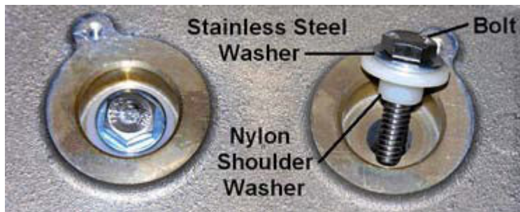
Figure 2-3: Insert ¼-in. Bolts
