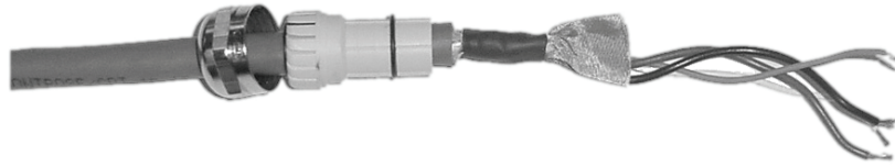
Figure 8 Applying the heat shrink
